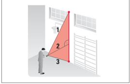
Press this button five times; the display shows the following symbol  $\angle$ . The laser is switched on.
