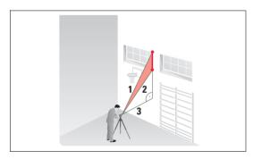
e.g. determining the height between point 1 and point 2 using three target points.
