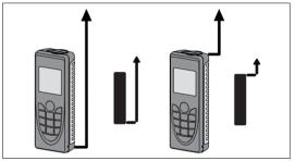
Press this button for longer and the front reference is set as default until unit is powered off.
