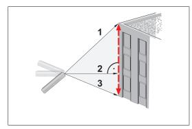
Press this button **twice**; the display shows the following symbol . The laser is switched on. Aim at the upper point (1) and trigger the measurement. After the first measurement the value is adopted. Keep the instrument as horizontal as possible
